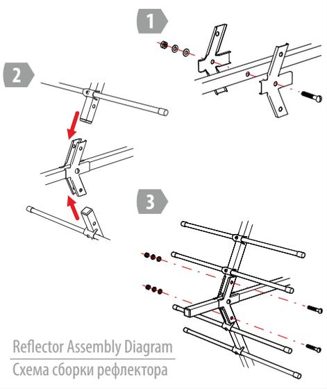
Reflector Assembly Diagram
